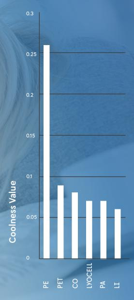
Q-max measures the highest value of heat transfer within 0.2 seconds after contact. The higher the Q-max value, the better the cooling effect.
